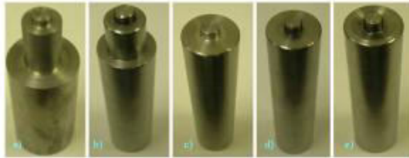
Figure 3: Various tool design used for FSW Process
